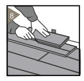
To lay the last row, place a full length floor board directly on top of the last installed row. Measure and cut the correct width by putting a full width scrap board with spacers inserted against the wall..
