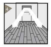
Boards shall run lengthwise against the longest wall. When possible try to run floor boards parallel to incoming sunlight or main light source.
