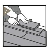
On the far wall, place a full length floor board directly on top of the last installed row. Measure and cut the correct width by putting a full width scrap board.
