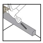
Make sure to remove all spacers once the laying procedure is completed. Skirting boards or moldings shall be fastened to the adjacent wall by nail or screw, overlapping the expansion gap allowance.
