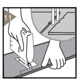
On encountering pipes, ensure the position and diameter of the pipe; drill hole(s) with diameter 3/8 in (10 mm) larger. Cut off as shown in the figure and lay the board in place. Apply adhesive to the loose piece and fit it in place.
