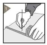
At each end of the starter wall, measure out the width of two boards plus the tongue and expansion gap allowance.
